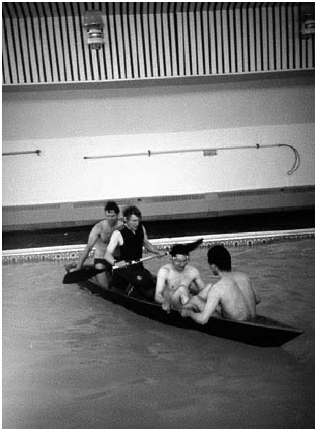
Floe edge boat experiment in the Igloolik community swimming pool to determine the seal-equivalent ballast limit of the prototype, 1985. Photo: John MacDonald
